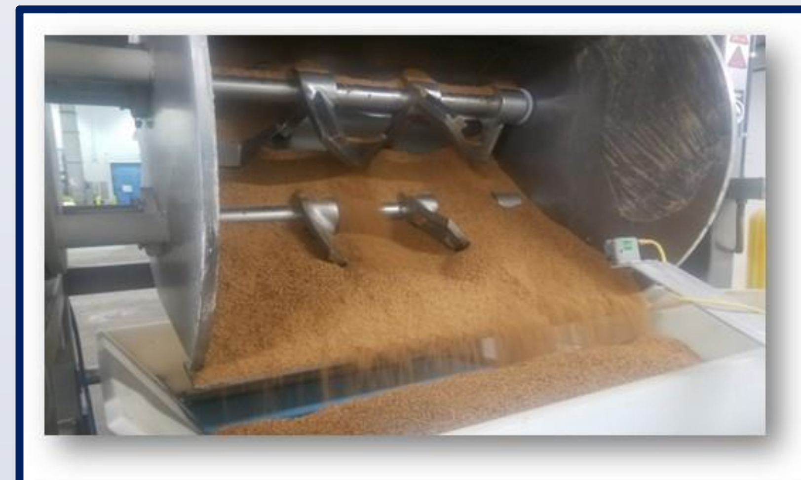
Purging with granola as an abrasive material
