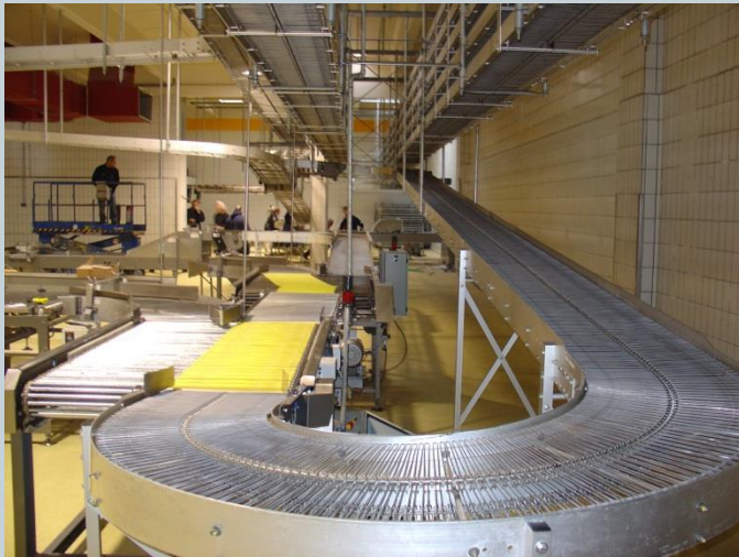
Continuous conveyor design minimizes product transfers
